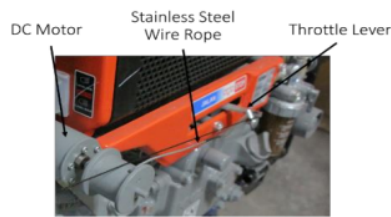
Figure 18. G3000 throttle lever mechanical modification
