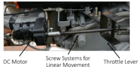
Figure 17. G1000 throttle lever mechanical modification
