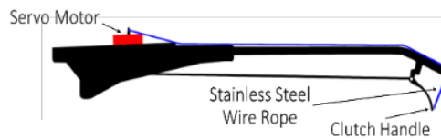
Figure 5. G1000 wire connection between servo motor and clutch handle design
