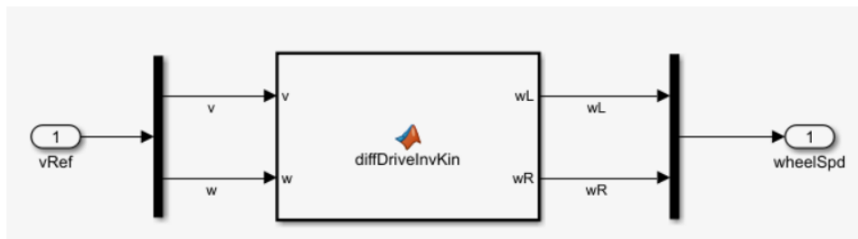
Figure 27. Differential drive inverse kinematics block detail
