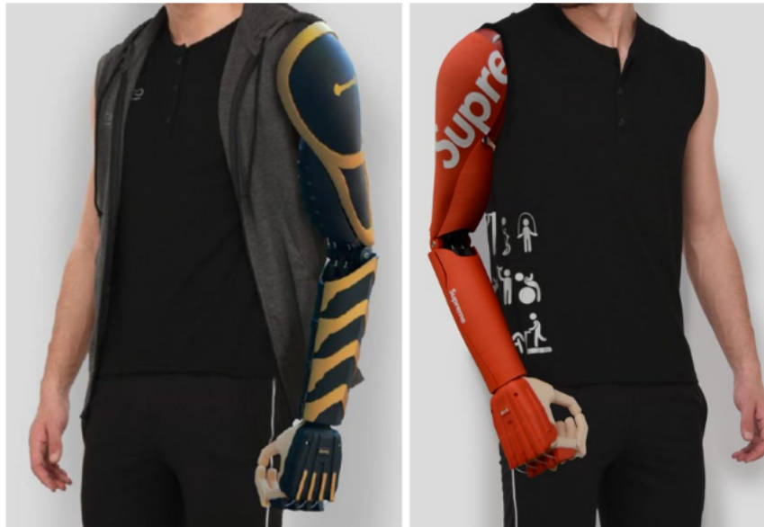
Figure 1. An example of an open-source shoulder disarticulation prosthetic design-based 3D printer that has been developed by iDIG Laboratory (Kuswanto et al., 2019)
